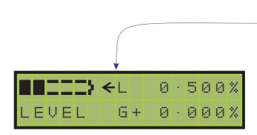
Indicates the direction laser beam is traversing and if left (L) or right (R) of centre. eg: Beam traversing left
