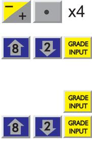
1. Enter the service program by operating the +/- switch once and the decimal point switch 4 times. Enter "1234" as a PIN using the keypad.
