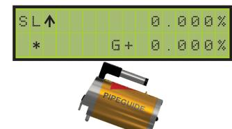
Self levelling at maximum Indicates the Pipeguide is tilted excessively upwards and needs to be lowered or positioned within range.
