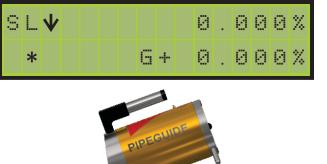
Self levelling at minimum Indicates the Pipeguide is tilted excessively downwards and needs to be raised or positioned within range.
