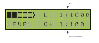
Indicates in ratio format the distance the line is to left (L) or right (R) of centre.
